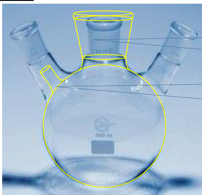
Figure 2 Modifications on 3-neck round-bottom flask
